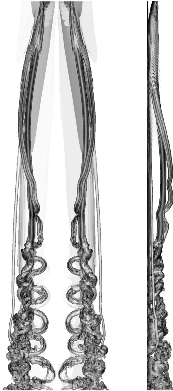
Fig. 19. 3-D space-developing LES of wake vortices behind an elliptically loaded wing in ground effect: isosurfaces of vorticity norm, \|\omega\|_{t_0} = 80 (opaque) and 25 (semi-transparent), colored by the longitudinal component of vorticity, when the flow has reached it's regime. Top and side views.
